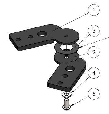
Friction pad glued in place with adhesive
